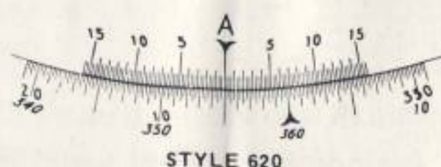
Circle graduated to 15 minutes. Verniers read directly to 20 seconds.
