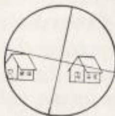
Fig. 12. Test of Horizontal Cross-hair of Dumpy Level
